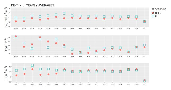
Note: in 2017 the ICOS setup has been implemented. Close path IRGA with 63m tube. PI processing using Eddypro
