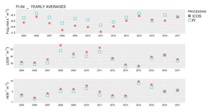
Note: in 2015 the ICOS setup has been implemented. Close path IRGA with 13m tube. PI processing using EddyUH
