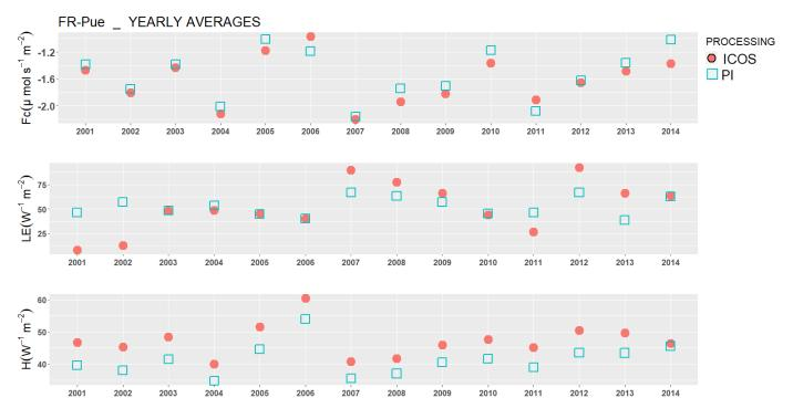
Note: in 2014 the ICOS setup has been implemented. Close path IRGA with 3.5m tube. PI processing using Eddypro
