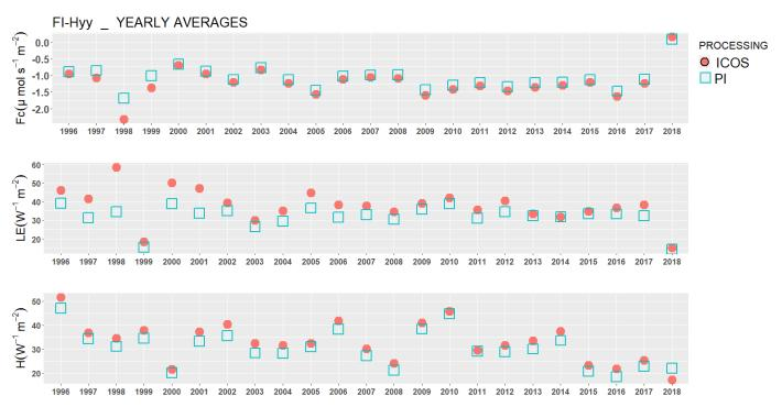
Note: in 2018 the ICOS setup has been implemented. Close path IRGA with 8m tube. PI processing using EddyUH
