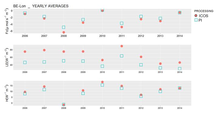
Note: in 2014 the ICOS setup has been implemented. Close path IRGA with 12m tube. PI processing using Eddysoft
