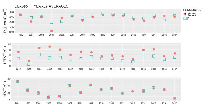
Note: in 2017 the ICOS setup has been implemented. Close path IRGA with 12m tube. PI processing using Eddypro
